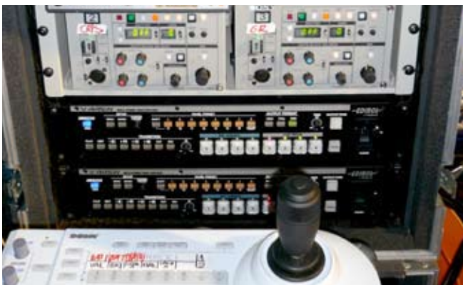
2 V-44SW Multiformat Video Switcher at CCU rack (Heroes del Silencio World Tour 2007)
