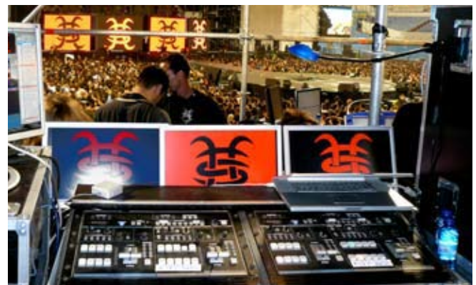
2 V-440HD MultiFormat video mixer at main video control (Heroes del Silencio World Tour 2007)
