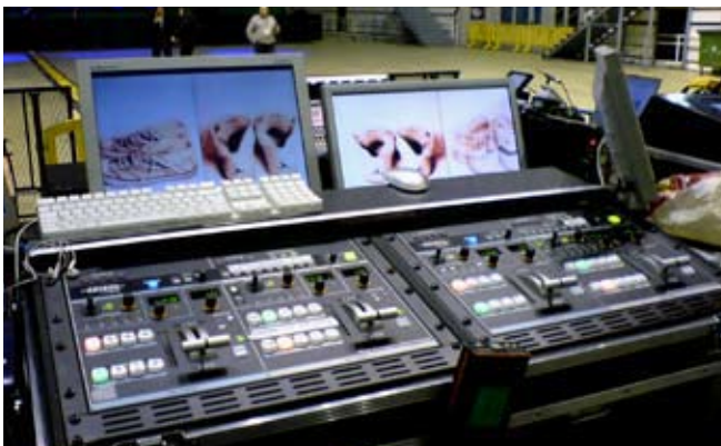
2 V-440HD MultiFormat video mixer at main video control (El canto del loco World Tour 2006)
